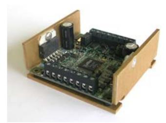
The development of proprietary circuits has minimized ripple current while maintaining a 25 KHz chopping rate.
